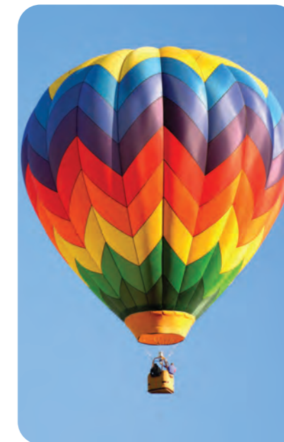
▲ Hot air is less dense than cold air, so a hot-air balloon will rise upwards – provided the fabric, gas cylinders, basket, and passengers do not increase the average density by too much.
